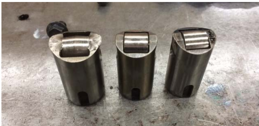
Figure 9 - large tappet on left, two small tappets on right Large tappet roller has seized.
