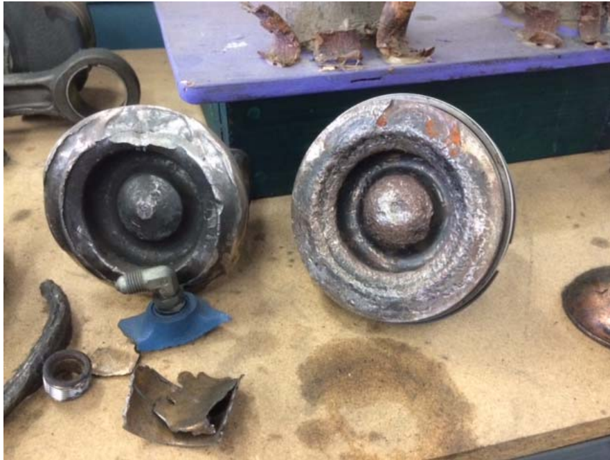
Figure 10 - damaged pistons due to internal engine failure
