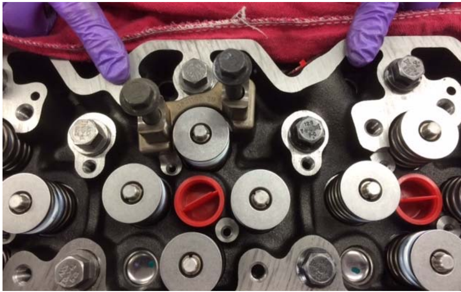
Figure 8 - close-up showing lack of oil channel on #5 cylinder Technician's purple-gloved fingers point to oil channel locations. Note the lack of a oil-channel on the left #5 cylinder. #6 cylinder on right.
