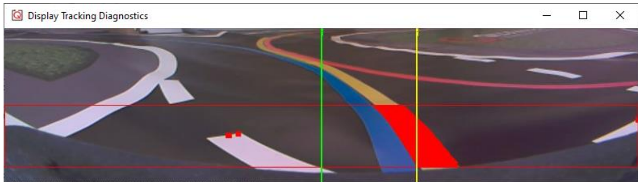
Figure 3. Processed lane extraction Image.
