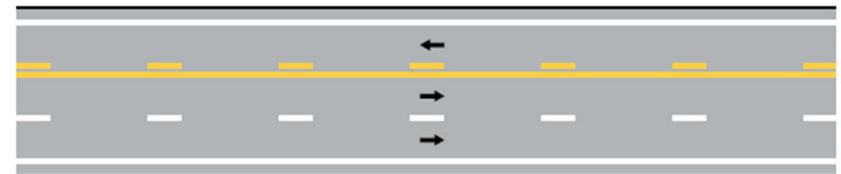
A – Three-lane, two-way marking with passing permitted in single-lane direction
