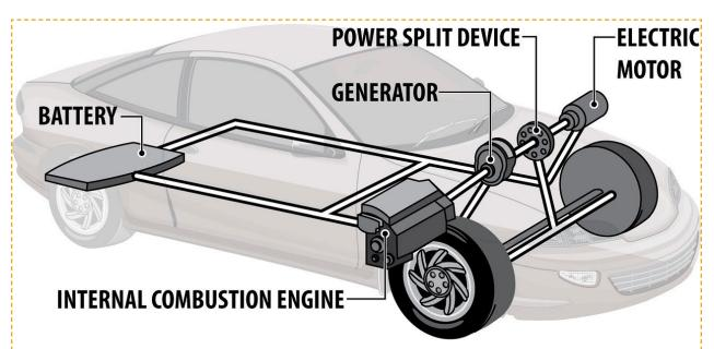
Hybrid electric vehicles combine the benefits of gasoline engines and electric motors. Typically, the wheels are powered by an electric motor, and in some cases, the internal combustion engine assists. Hybrid electric vehicles do not need to be plugged in to charge the battery because they are charged by an onboard generator.
