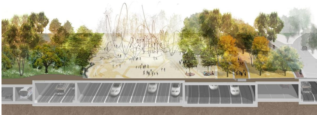
Figure 95. El Parc del Camí Comtal buries rail and road infrastructure and brings 180,000 locals new access to a new expansive urban park. Source: BSAV
