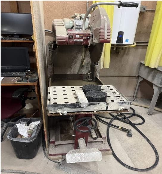
Figure 9. Saw-Cutting Specimen Along its Edge
