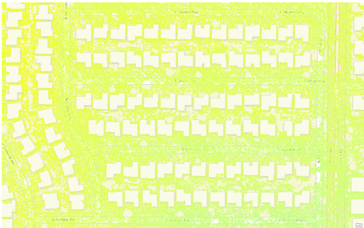
Figure 4. Example of Ground Points in Point Cloud Data
