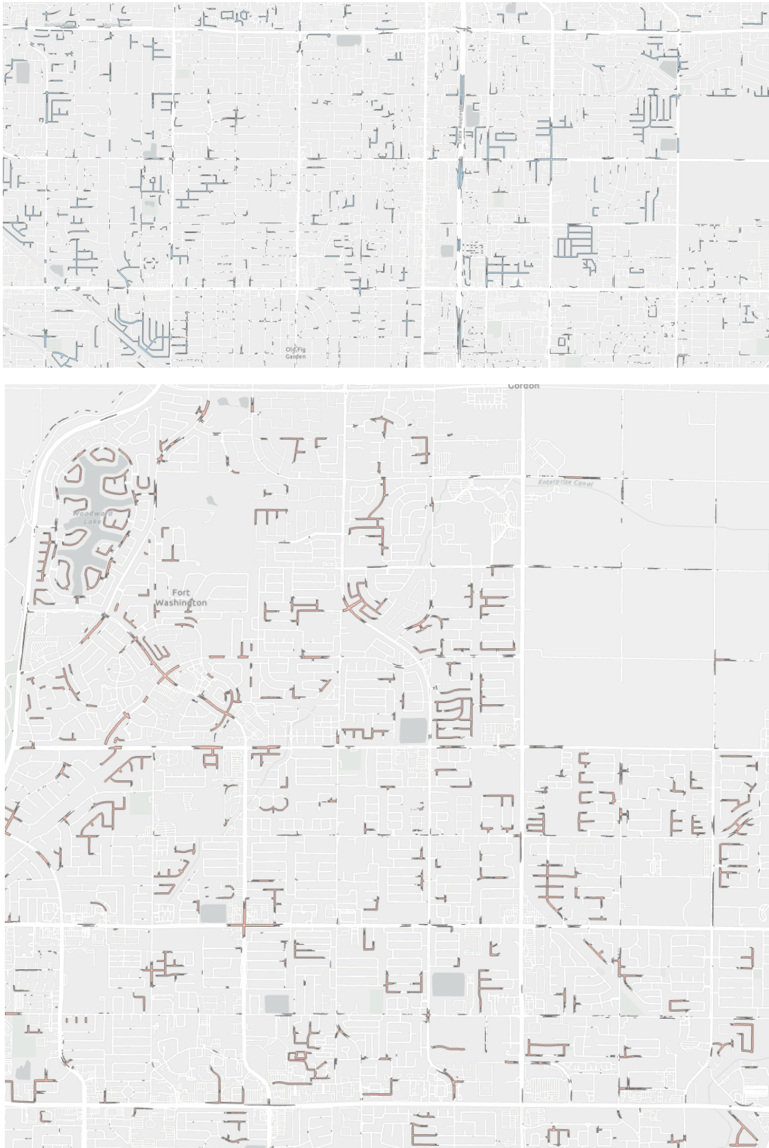
Figure 20. Road Intersected Ponding Polygon
