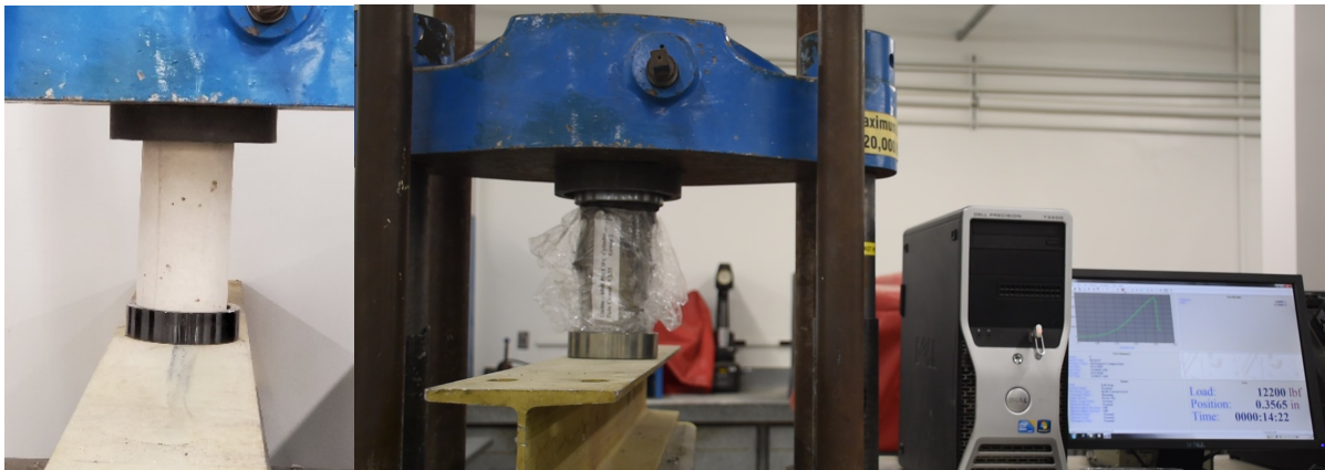
Figure 22. Compressive Strength Sample (Left) and Testing (Right)
