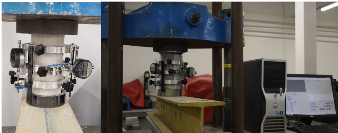
Figure 23. Static Modulus of Elasticity Test Sample (Left) and Testing (Right)
