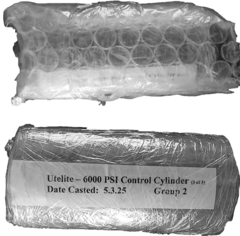
Figure 21. Protecting (Top) and Sealing (Bottom) Samples
