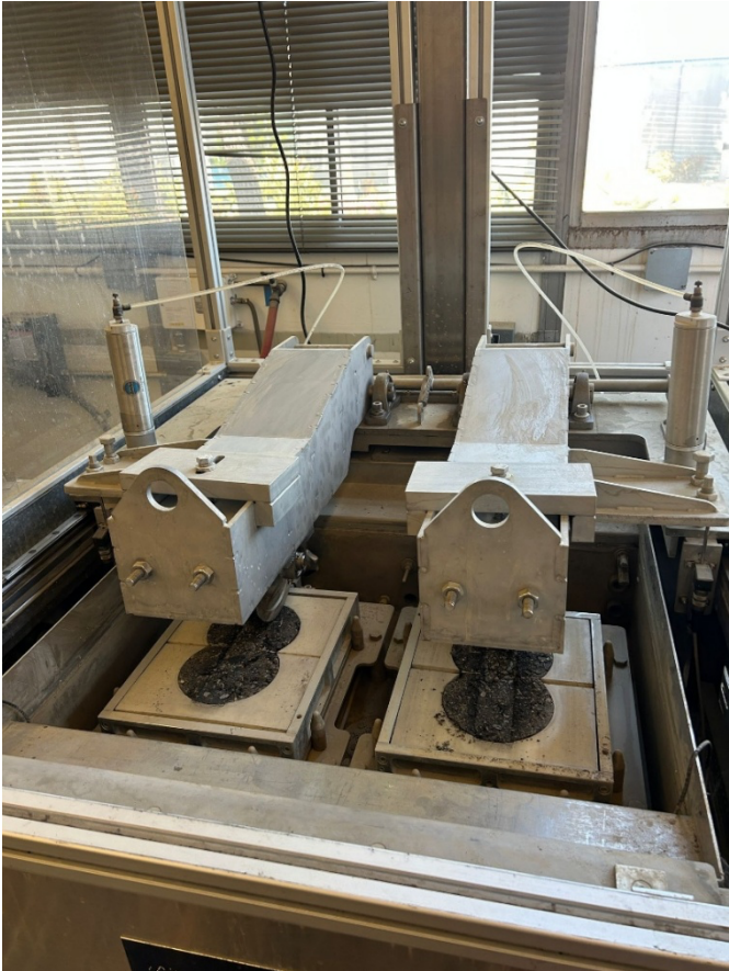
Figure 9. Hamburg Wheel Track Test Setup After Test
