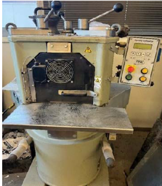
Figure 7. Superpave Gyrotory Compactor for Specimen Compaction
