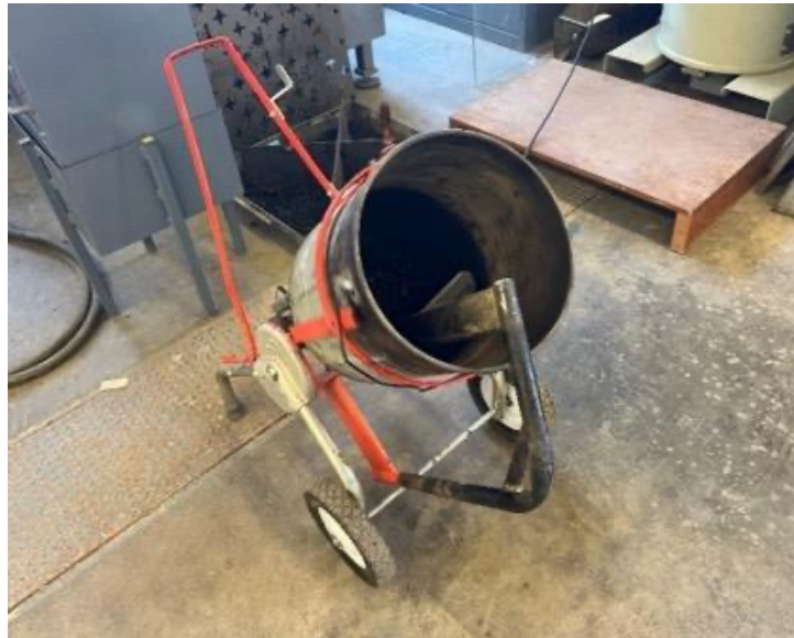
Figure 4. Mobile Mixer to Mix Aggregates with Binder
