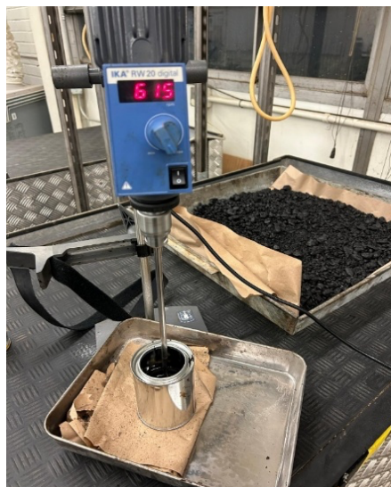
Figure 2. Shear Mixer Used for This Project
