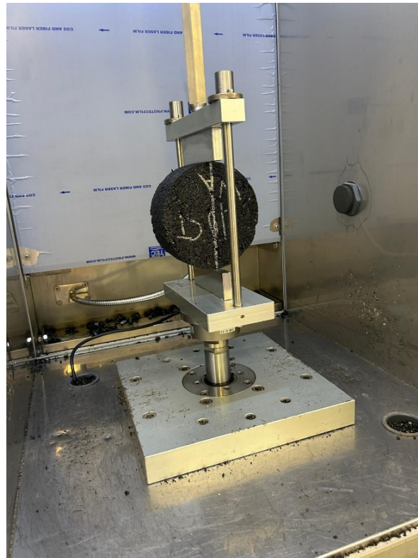
Figure 8. DTS Machine for IDEAL-CT Testing
