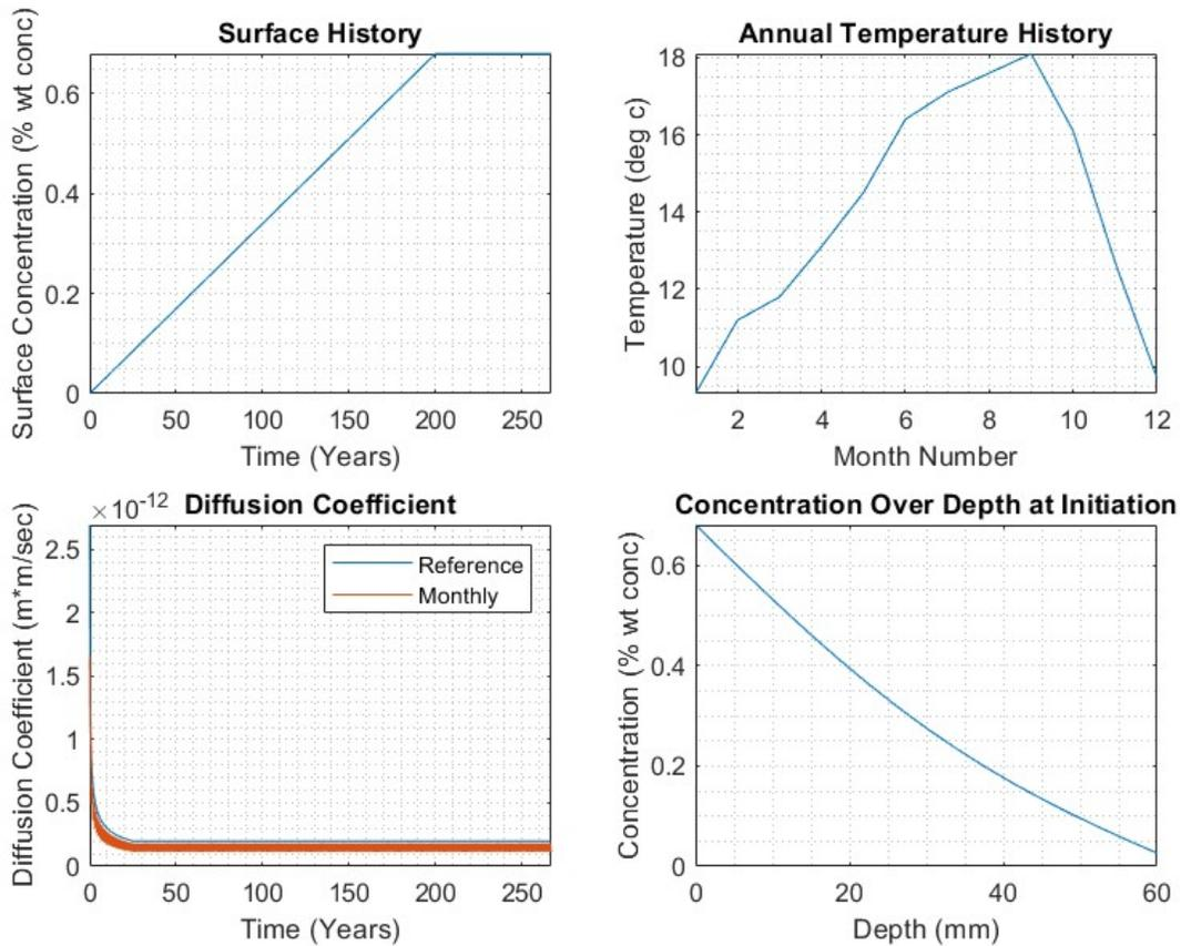
Various material properties and climate conditions influence the predicted service life of concrete. Therefore, when comparing the service life of different concrete specimens, it is important to relate them to the service life of a witness sample tested in the same climate. Consequently, the varying trends in predicted service life, based on diffusion coefficients, shown in Figure 53, are affected by the specific locations where these measurements are taken.
