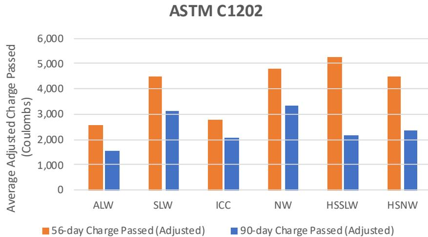
Figure 44 clarifies observations using normalized average values related to the normal weight concrete witness specimens. The results indicate that lightweight aggregates reduce the adjusted passed charges by 22 to 52 percent for normal-strength concrete at 56 days and 7 to 38 percent at 90 days. Additionally, the High-Strength Self-Consolidating Lightweight Concrete (HSSLW) shows an 18 percent increase at 56 days, decreasing to an 8 percent reduction at 90 days.
