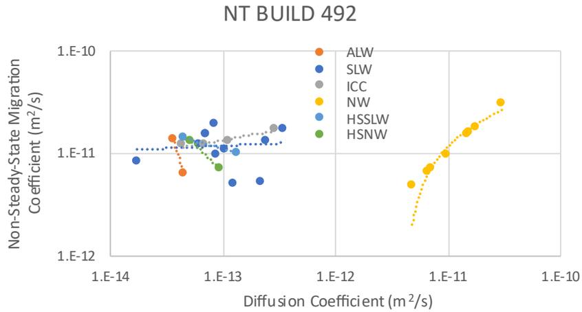
Figure 48 compares the chloride migration and diffusion coefficients. The graphs indicate that the diffusion coefficients derived from the charges passed suggest a trend of decreasing diffusion over time for all concrete specimens. However, this trend is not evident for the migration coefficient, except in the NW specimen.
