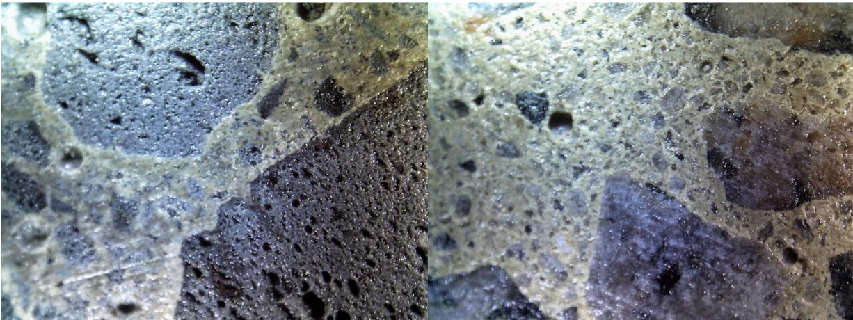
Figure 23. Cut Surfaces of Internally Cured (Top-Left), Sand-Lightweight (Top-Right), and Normal-Weight (Bottom) Concrete Samples
