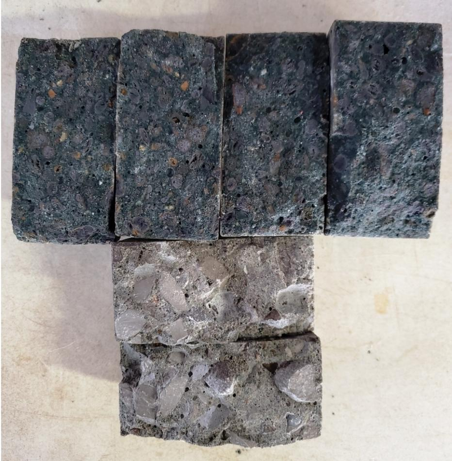
Figure 22. Magnified Views of All Lightweight (Left) and Normal-Weight (Right) Concrete Samples
