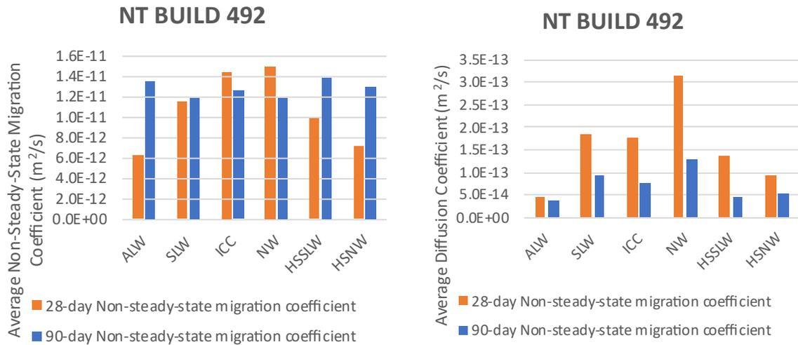
The normalized ratios in Figure 50 indicate that concrete containing lightweight aggregate has a slightly higher migration coefficient compared to the normal-weight control specimens. However, the impact of the lightweight aggregate is reflected in the reduction of the diffusion coefficient, which varies from 13 to 58 percent, except in a single case involving HSSLW at 28 days.
