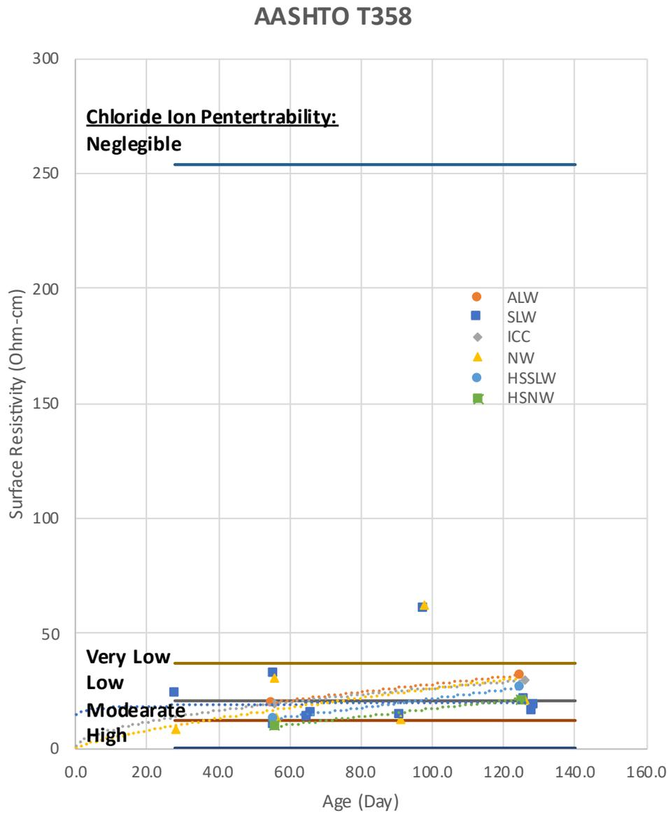
Figure 36 compares the results for ages 28 and 90 days, indicating a considerable increase in surface resistivity of 78 to 220 percent. The increase was significantly higher for high-strength concrete specimens than for normal-strength concrete specimens.
