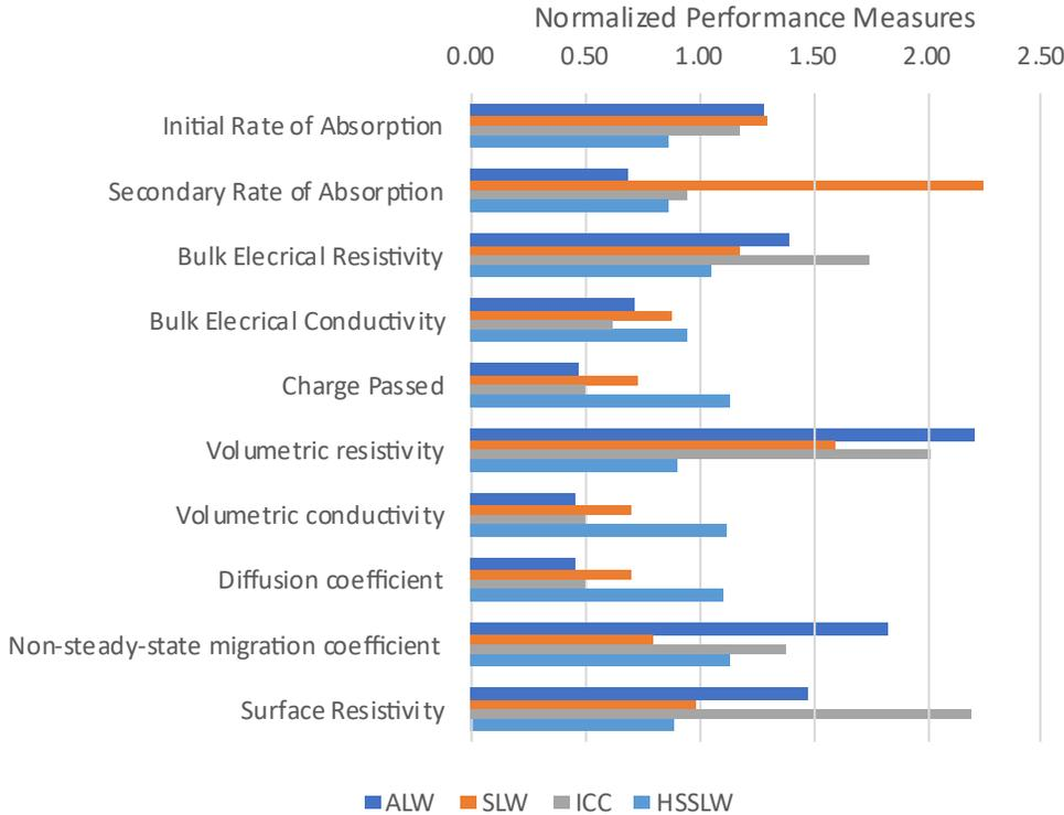
Lightweight aggregates significantly enhance the service life of concrete while also reducing lifecycle costs and greenhouse gas emissions. Figure 63 indicates that the long-term performance of concrete made with lightweight aggregates far outweighs any modest increases in cost or greenhouse gas emissions associated with the production and construction of these materials.
