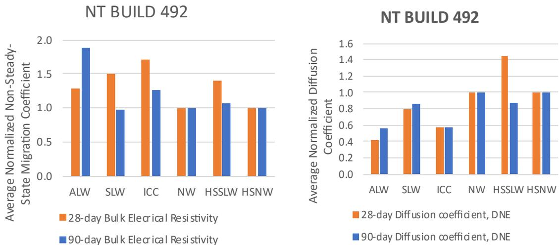
The diffusion coefficients from NT Build 492 are comparable to ASTM C1202, but this is not true for the migration coefficient, except for NW concrete (Figure 51).
