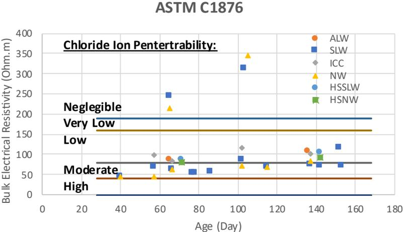
Figure 32 compares the results for 28- and 90-day ages, showing an increase in bulk electrical resistivity with age ranging from 22 to 41 percent, except for four data points that exhibit negligible chloride ion penetrability.
