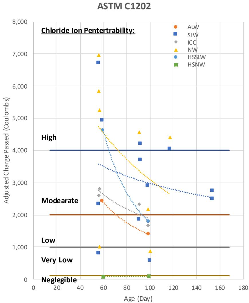
Figure 43 compares the average charges for all specimens, highlighting a decrease in observed values over time. The figure shows that the values for HSSLW are significantly higher at earlier ages but drop sharply as the ages increase. This suggests that there may be an issue with the samples tested earlier.
