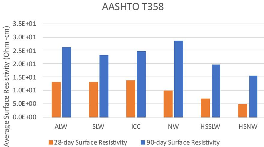
Figure 37 illustrates the impact of lightweight aggregates by comparing the surface resistivity of concrete that contains these aggregates to that of normal-weight concrete through normalized ratios. The results indicate that lightweight aggregates improve surface resistivity at 28 and 90 days, with enhancements ranging from 42 to 55 percent.
