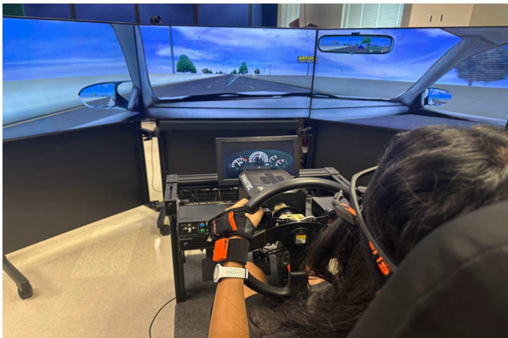
Figure 1. Demonstration of the Driving Simulator, Motion Capture System, and the Eye Tracking System During One Driving Trial
