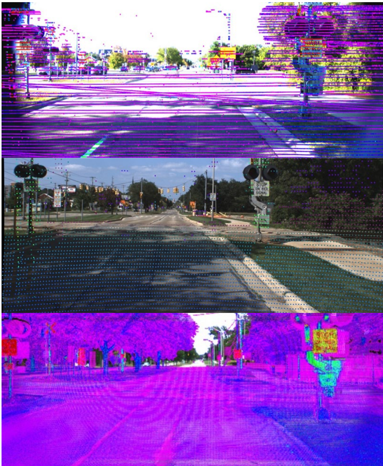
Figure 8. Point-cloud 3D lidar frames captured by different lidar sensors at different temporal frame rates of the same location around a railroad crossing.
