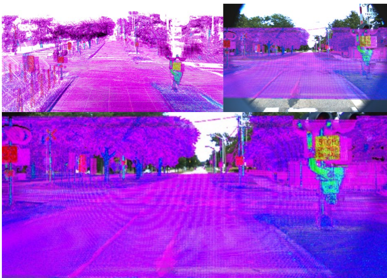
Figure 7. (Top left) high-resolution 3D point-cloud frame of a railroad-crossing scene captured by a Next Generation (NG) lidar used by the MSU team. (Top right) The fusion of the lidar point-cloud frame with the corresponding RGB camera frame. (Bottom) A zoomed-in version of the same scene illustrating the high-resolution features captured by the lidar to the extent that one can read the text “STOP” on the traffic sign at the railroad crossing.
