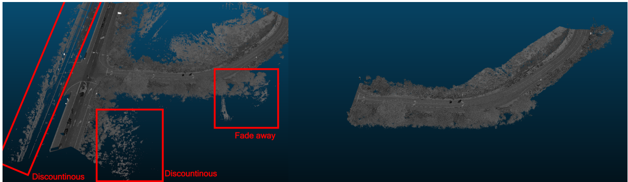
Figure 35. Example of Manual Filtering Pre-Process. Left Panel Indicates Area of Filtering and Right Panel Shows the Results After Filtering
