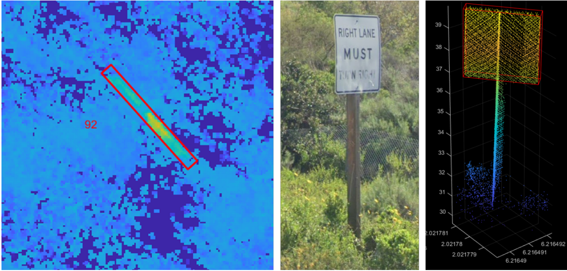
Figure 15. High Intensity Rectangle Feature (Left), Actual Traffic Sign (Middle), and Extracted Point Cloud (Right) for Five Signs
