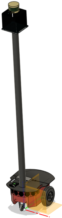
Figure 12. Smart Traffic Light Robot 3D CAD Model.
