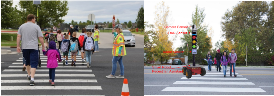
Figure 1. (a) School Personnel Helping Students Cross the Street, (b) Proposed Smart Robot Assisting Pedestrians Crossing the Street. The robot is mounted with several sensors and a traffic signal
