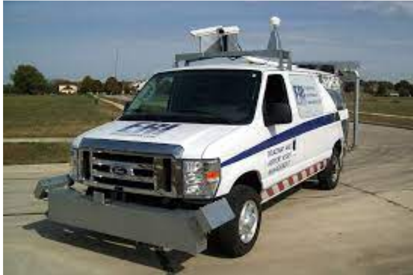
Figure 1. Vehicle Equipped with IRI Measuring Instruments
