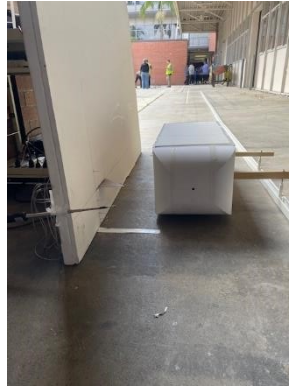
Figure 5. The Field Test With the Ahmed Body
