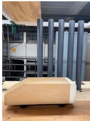
Figure 1. The Ahmed Body and the Vertical Columns
