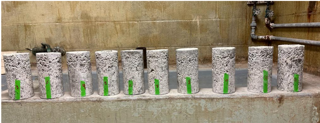
Figure 1: Cylinder Concrete Samples
