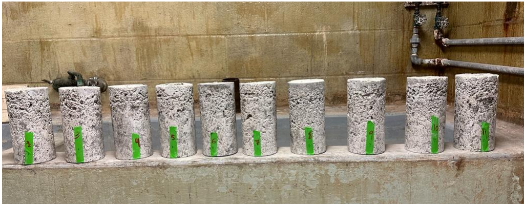
Figure 1: Cylinder Concrete Samples
