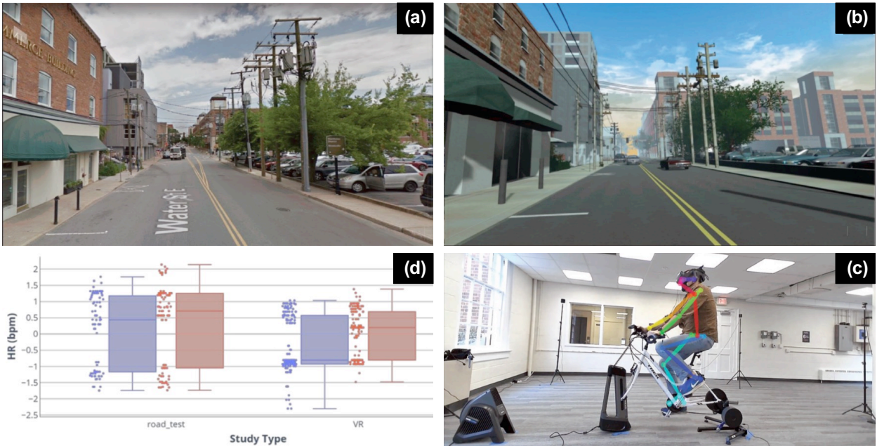
Figure 2. Comparison of (a) Real Road and (b) IVE Environments; (c) Video Collection System of IVE Bike Simulator; (d) Heart Rate Distribution of Experiment
