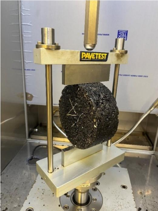
Once the load versus displacement graph was generated, the work of failure ( $W_f$ ) was determined by calculating the area under the load versus displacement curve using the quadrangle rule, as shown in the equation below:
