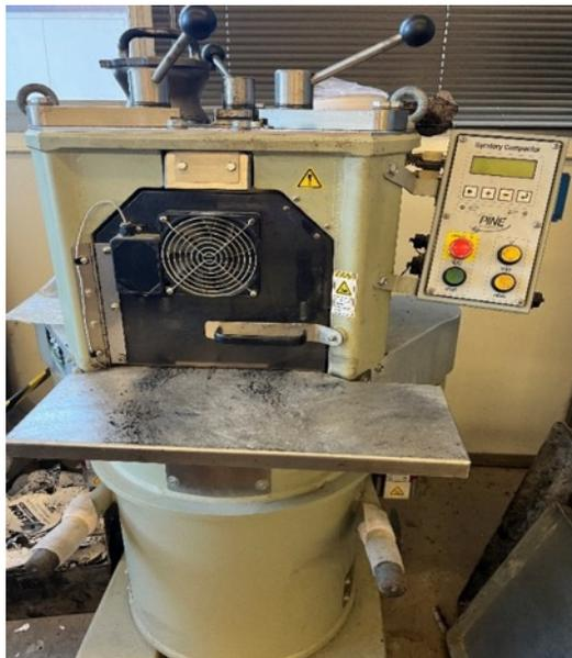
Once compaction and squaring of the samples were completed, the compacted specimen was extruded and allowed to cool to room temperature as illustrated in Figure 10. Each specimen was appropriately labeled for identification. Subsequently, after reaching room temperature, the bulk specific gravity ( $G_{mb}$ ) of each specimen was determined.
