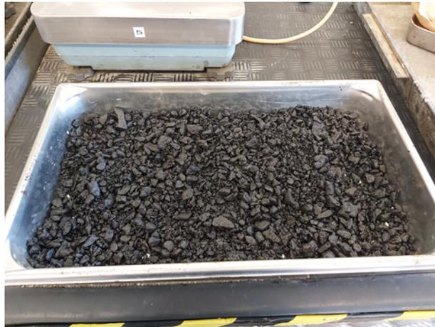
The pans were then placed into the forced draft oven set at  $95 \pm 3^\circ\text{C}$ , as shown in Figure 7. In this procedure, the required duration of aging to simulate the desired field aging was determined using the following equation:
