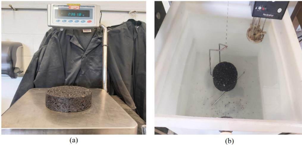
Once the  $G_{mm}$  and the  $G_{mb}$  were determined, the AASHTO T 269 test method was employed to calculate the air voids ( $V_a$ ) in the compacted HMA samples using the formula:
