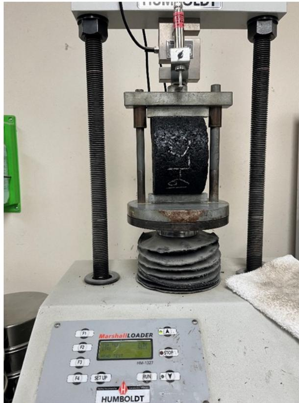
The indirect tensile strength (ITS) for each specimen was calculated using the following equation:
