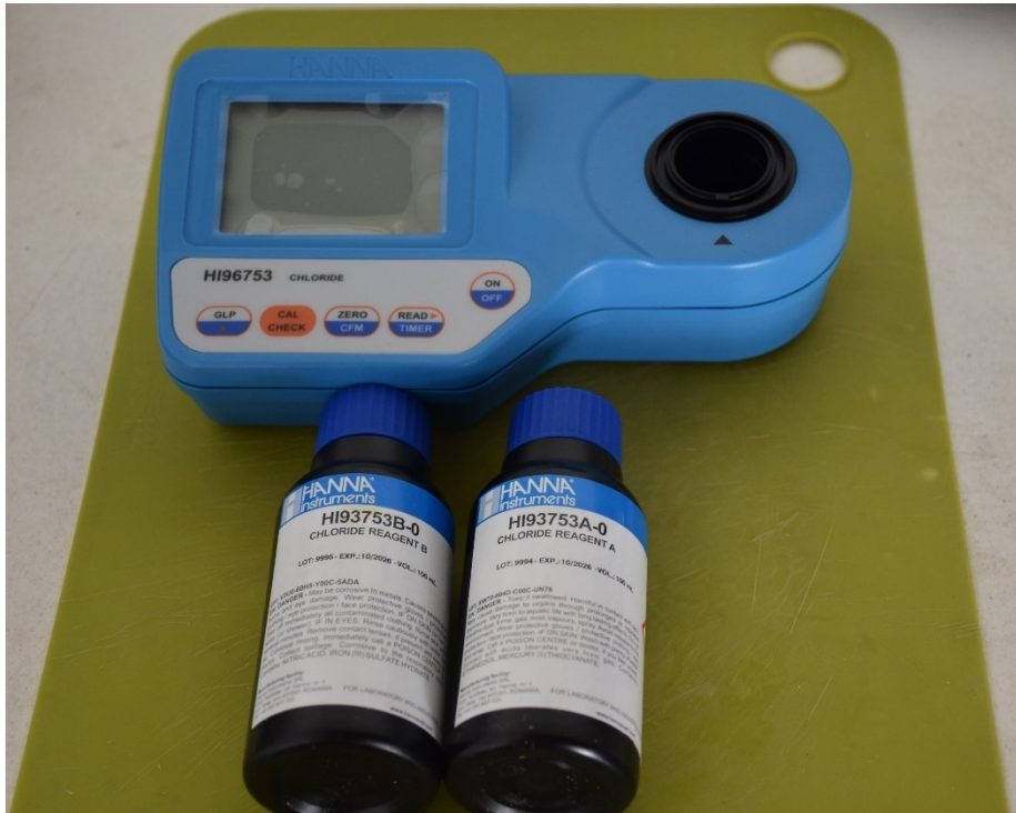
Figure 21. Chloride Photometers and Reagents
