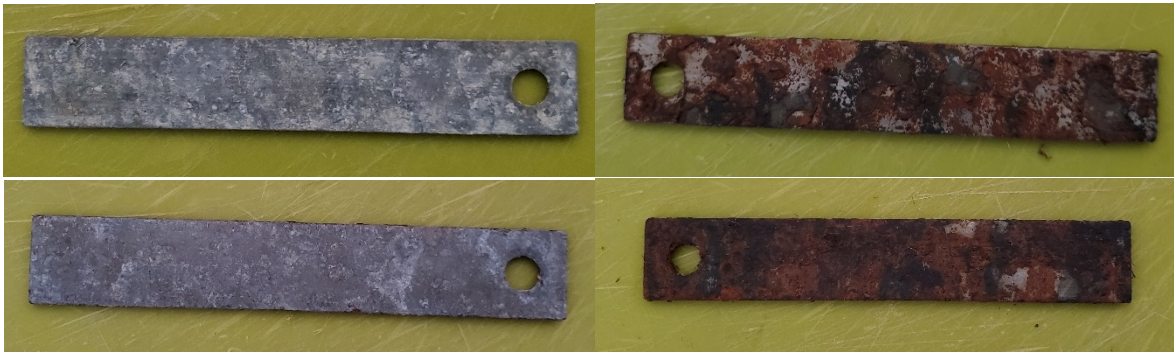
Figure 76. Examples of Galvanized (Left) and Carbon (Right) Steel Coupons Corrosion Embedded in Normal Weight (Top) and Lightweight (Bottom) Aggregates
