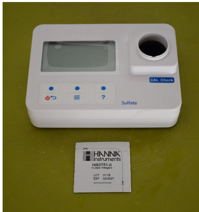
Figure 20. Sulfate Photometers and Reagent
