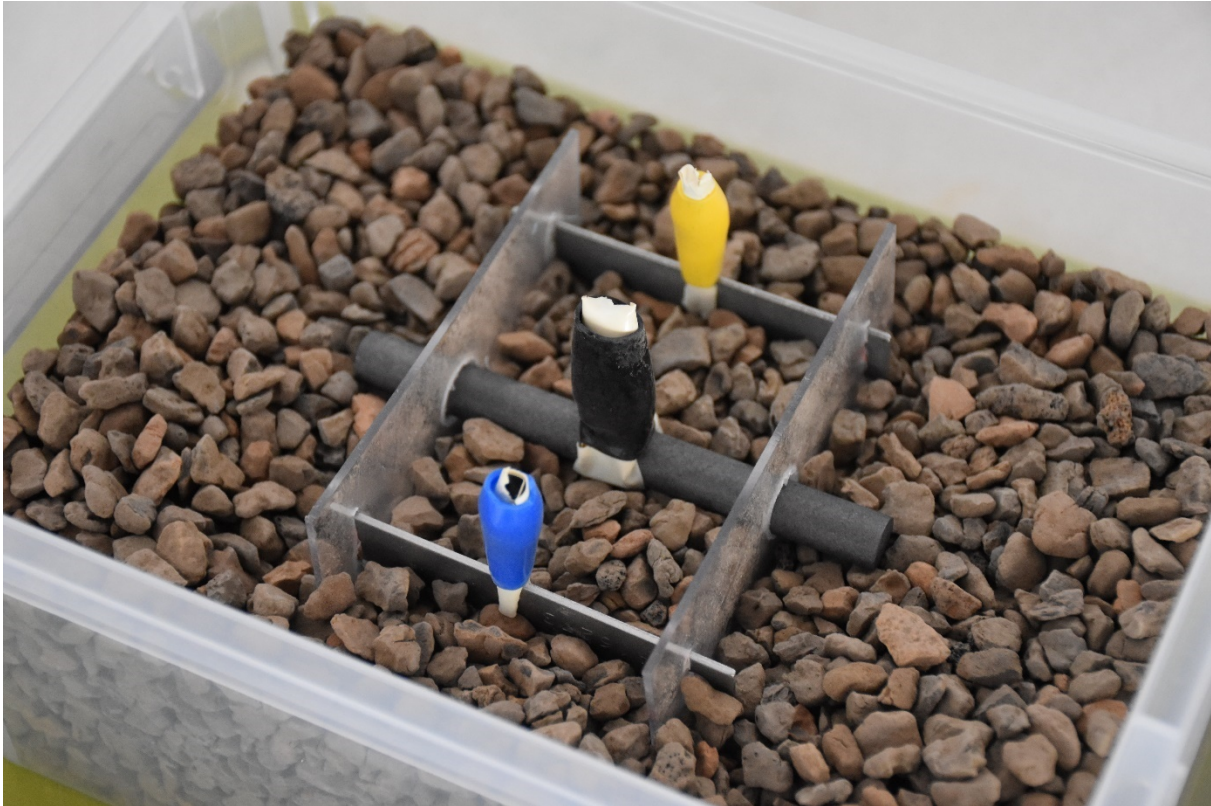
Figure 25. Arrangement of Galvanized (Yellow Connector) and Carbon (Blue Connector) Steel Coupons as Working Electrodes and Reference Counter Electrode (Black Connector) Before Burial into Aggregate Samples
