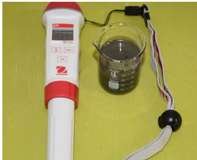
Figure 17. The pH Meter and a Sample Solution
