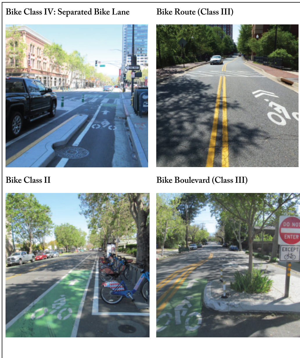
Figure 4. Examples of Different Bike Lane Classes from San José, CA (City of San José Department of Transportation, 2020)
