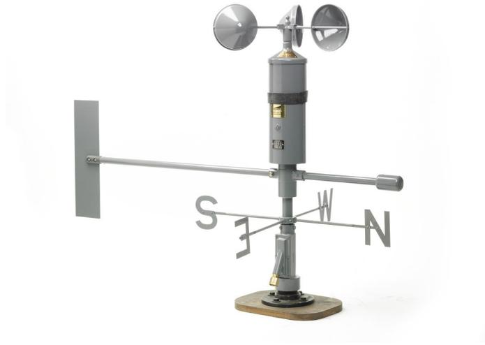
Figure 2.17. Conventional anemometer mounted on a pole for wind speed measurement (source: munroinstruments.com).
