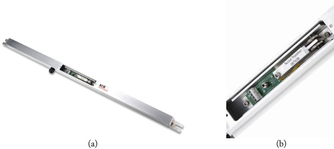
Figure 2.14. a) A tilt beam rotational sensor, b) a zoomed in view of the tilt sensor at the center of the casing rod (source: soilinstruments.com).
