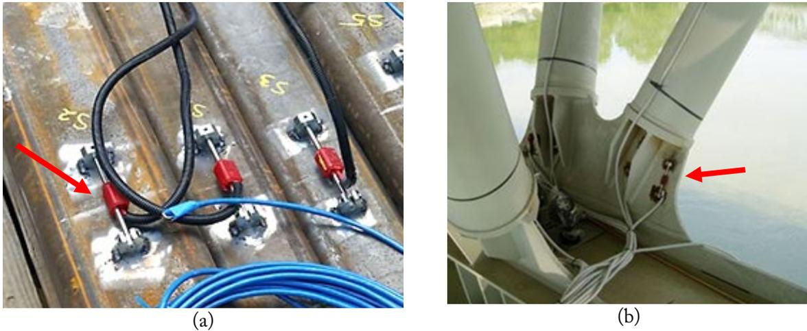
Figure 2.8. Examples of vibrating wire strain gages for monitoring steel structures. a) steel profile with welded VW strain gages (source: geo-instruments.com), b) VW strain gages attached to steel joint plates of a bridge (source: spectotechnology.com).
