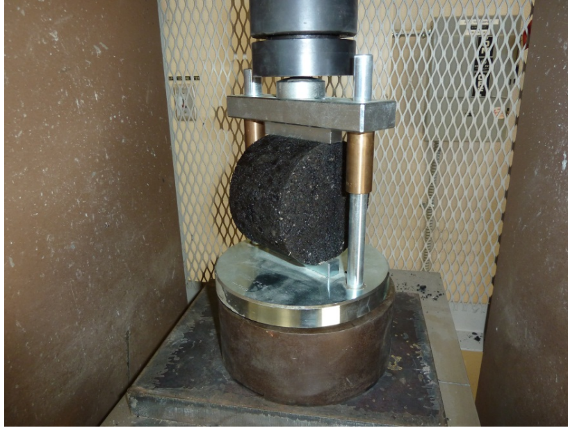
Figure 14. Specimen after Indirect Tensile Test
