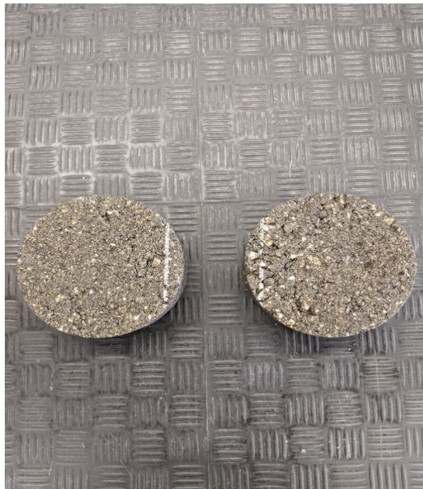
Figure 5. Marking of Cut Line of PG 70-22 and G5 Mix for Hamburg Wheel Tracking Test
