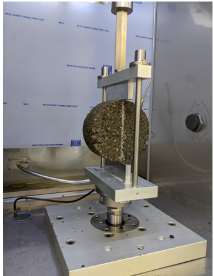
Figure 1. G5 sample during IDEAL Cracking Test.
