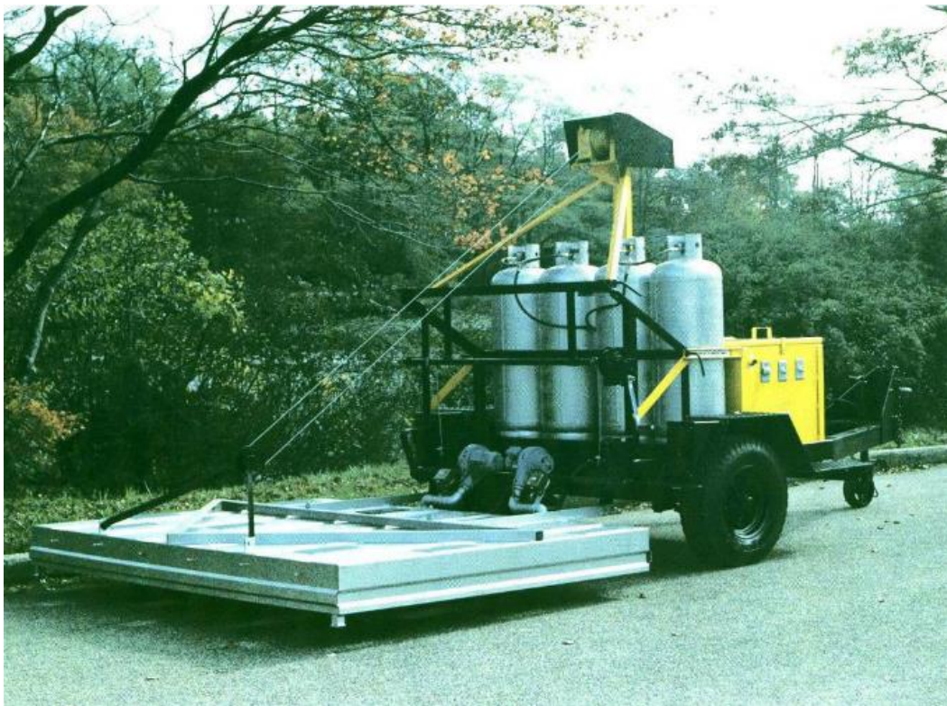
b. Heater Patching Trailer
