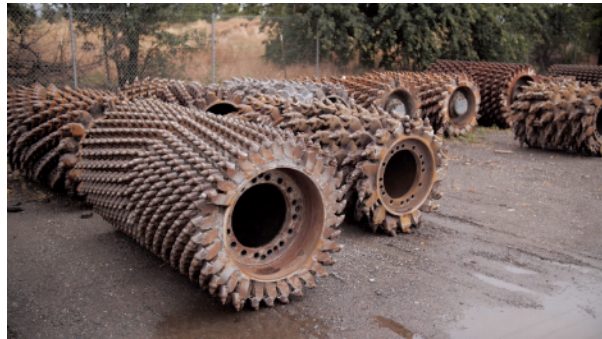
a. Micro-milling Drum in Foreground
