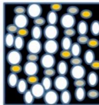
Particulates are brought together by removing voids at high compression. Increases the effective volume fraction. For 93.5 – 99 % increase in  $V_f$ , this increases stiffness  $E$  from 0.5 – 100 MPa ( $E_{gravel}$  is 100 GPa) .
