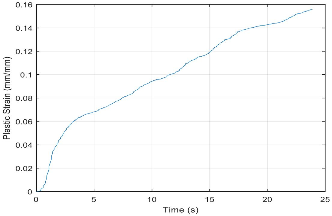
Figure 20. Plastic Strain Wear Rate for CFRP
