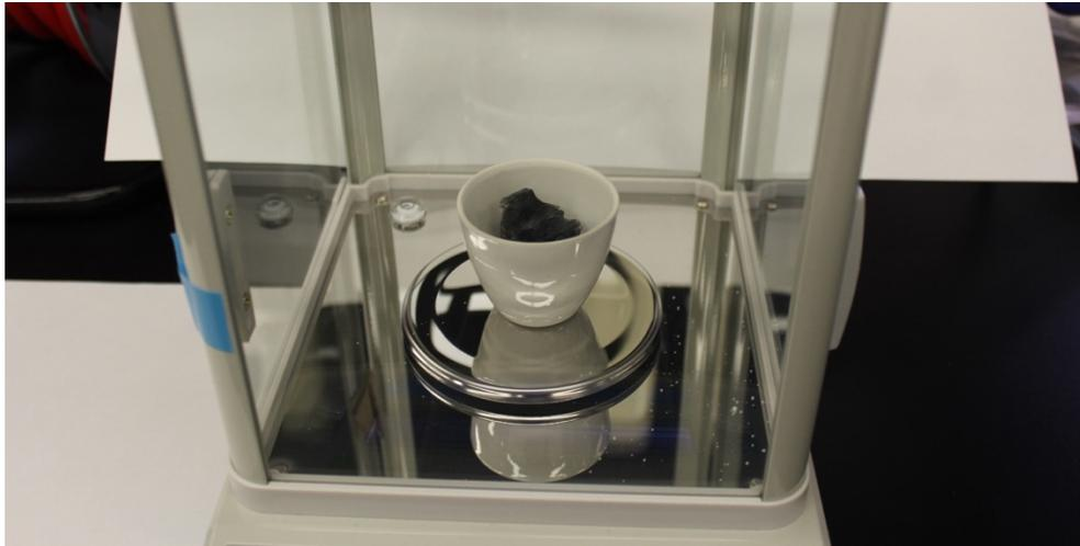
Figure 4. High Temperature Burnoff Following ASTM D 3171 – A7
