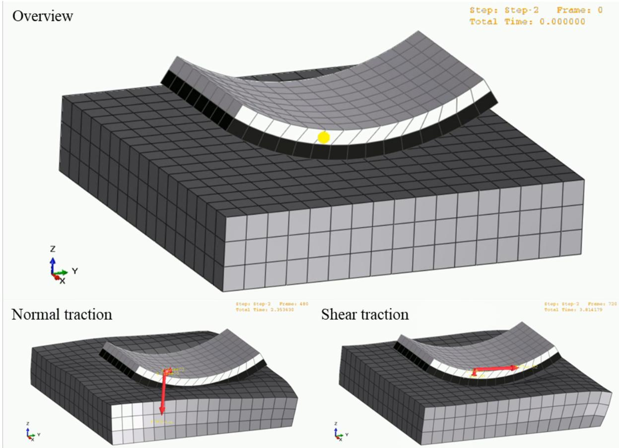
Figure 22. Comparison of Stress and Deformation of Asphalt Versus Composite
