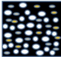
Gravel particulates can freely move in the bitumen binder. Volume fraction  $V_f$  is preserved including voids.
