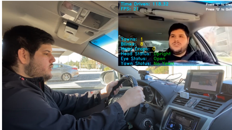
Figure 17. Live Demonstration of the Drowsy Driver Detection System in a Vehicle.
