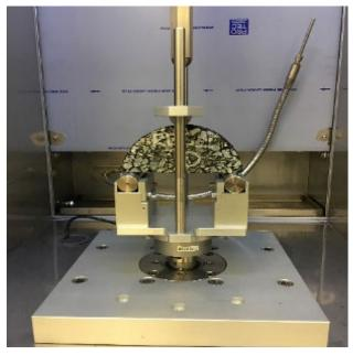
Figure 1. SCB Samples During Testing
