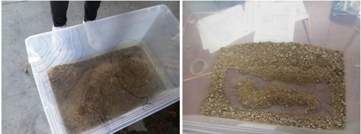
Figure 22. Design of Topographic Maps and Earthwork Quantity Estimations
