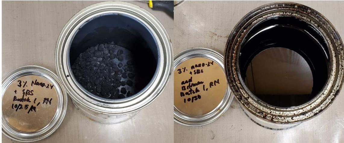
Figure 1. Fully Dried 3% Nano-24-Coated SBS (left) & Heated Modified Asphalt Binder of 3% Nano-24-Coated SBS + PG64-10 after using a High Shear Mixture (right)
