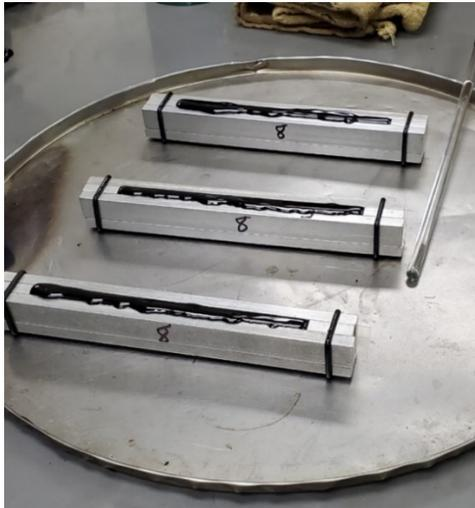
Figure 3. Specimen Molds with Modified Bitumen for the Bending Beam Rheometer Test
