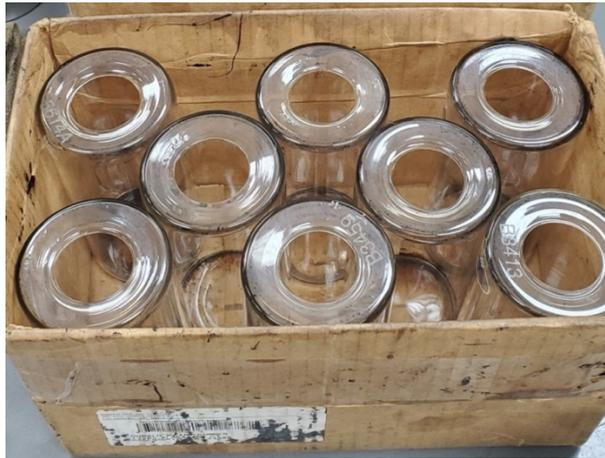
Figure 6. Rolling Thin Film Oven Cylinders
