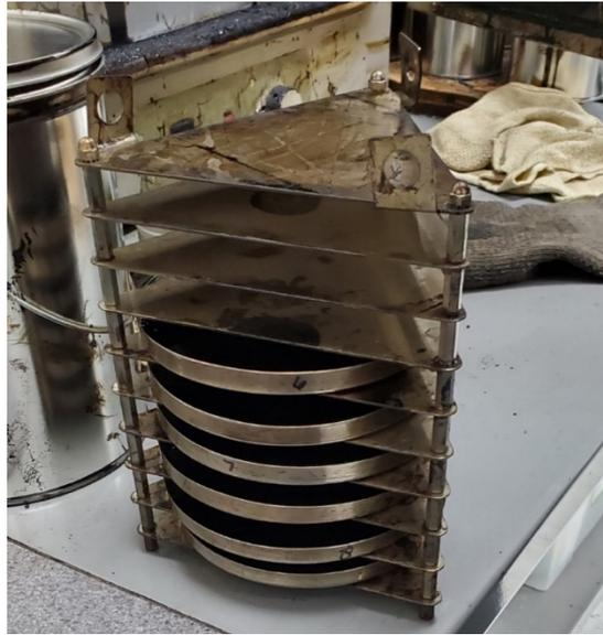
Figure 5. Thin Film Oven Pans for Pressure Aging Vessel Testing
