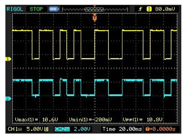
Figure 24. Transmitter and Receiver Voltage Captured On the Oscilloscope:
