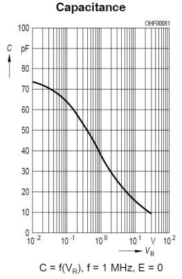
Figure 6. BPX61 Photodiode Junction Capacitance as a Function of Reverse Bias Voltage
