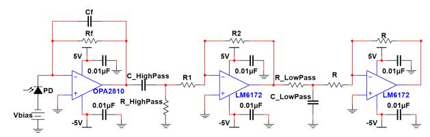
Figure 4. Photodiode Receiver Circuit
