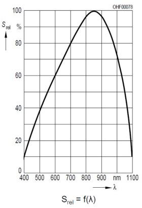
Figure 5. BPX61 Photodiode Relative Spectral Sensitivity as a Function of Wavelength
