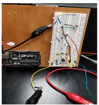
Figure 21. Receiver Circuit Design on Breadboard
