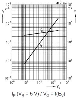
Figure 7. BPX61 Photodiode Photocurrent and Open-circuit Voltage as a Function of Luminosity
