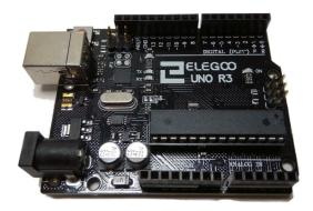
Figure 18. Arduino Uno R3 Board
