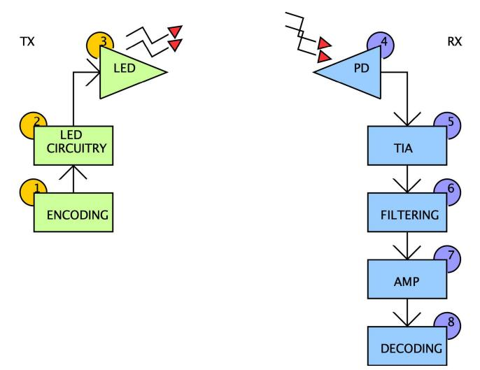
Figure 2. Block Diagram of VLC System
