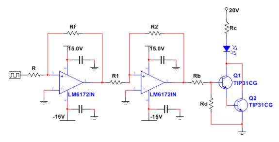
Figure 3. LED Driver Circuit
