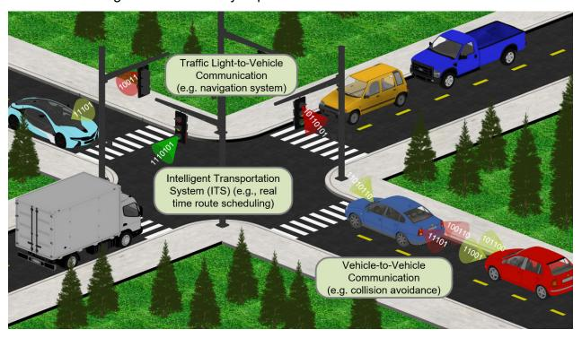
Figure 1. Intelligent Transportation System Using VLC Framework
