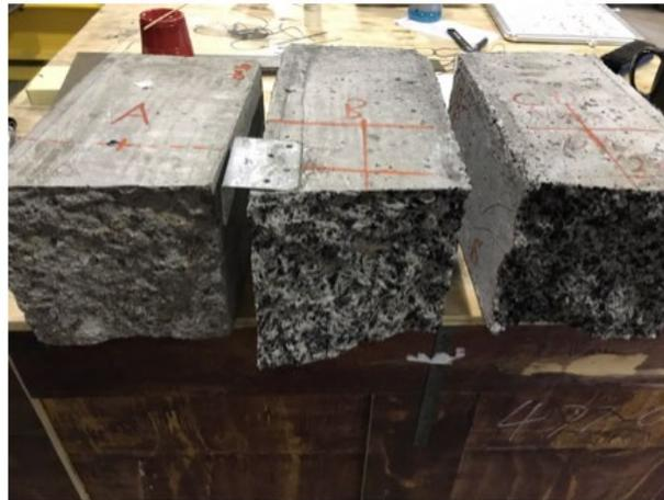
Fracture Surface of Beams with MIX A, B, and C
