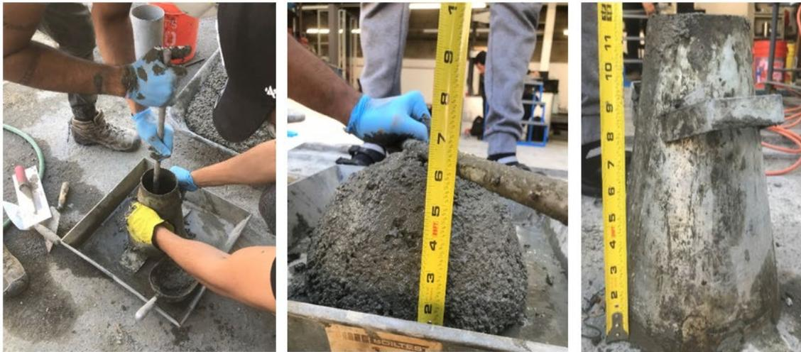
Slump Test (an average slump of 6–7 in. was reported for different mixes)
