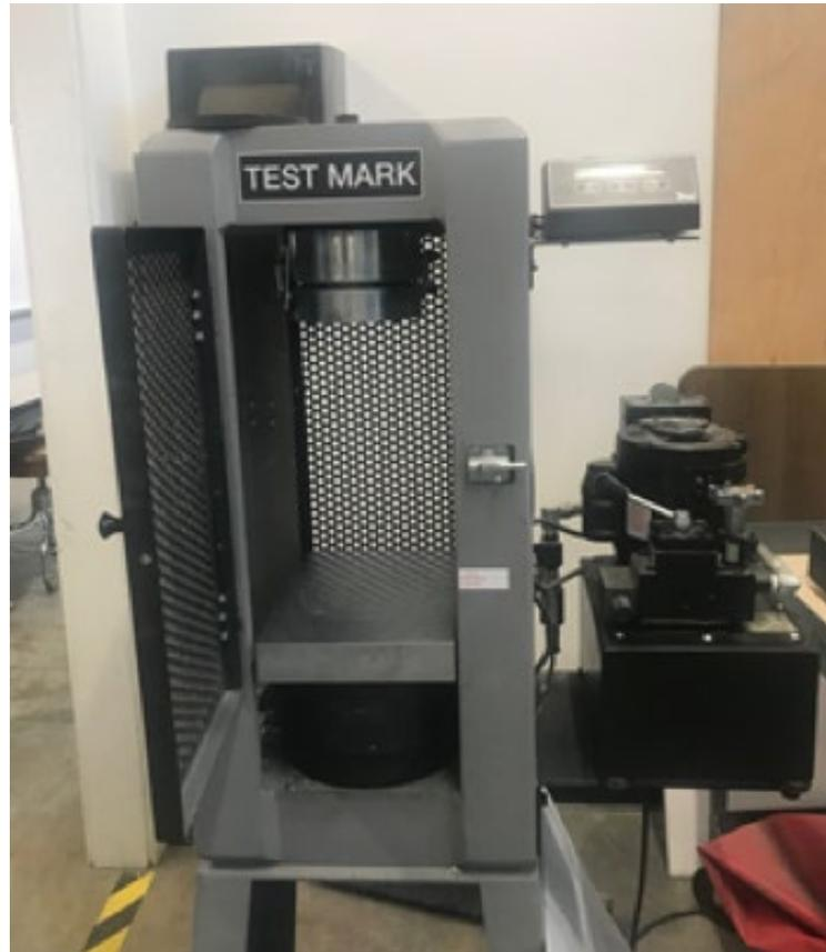
**Figure 5. Universal Testing Machine (UTM) for Materials Testing**
