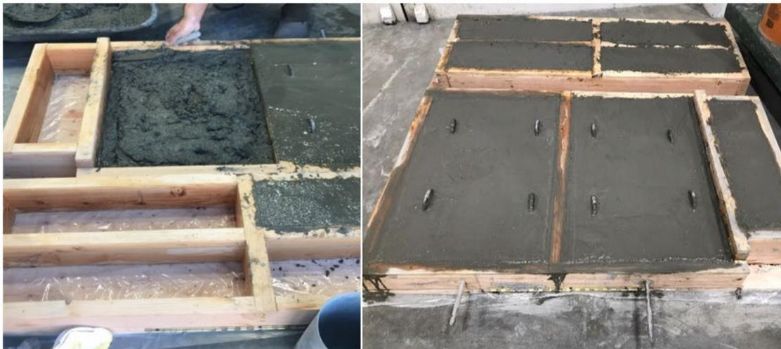
Fabricated concrete specimens
