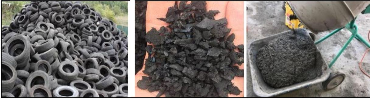
**Figure 1. Tire-Derived Aggregate Concrete**
