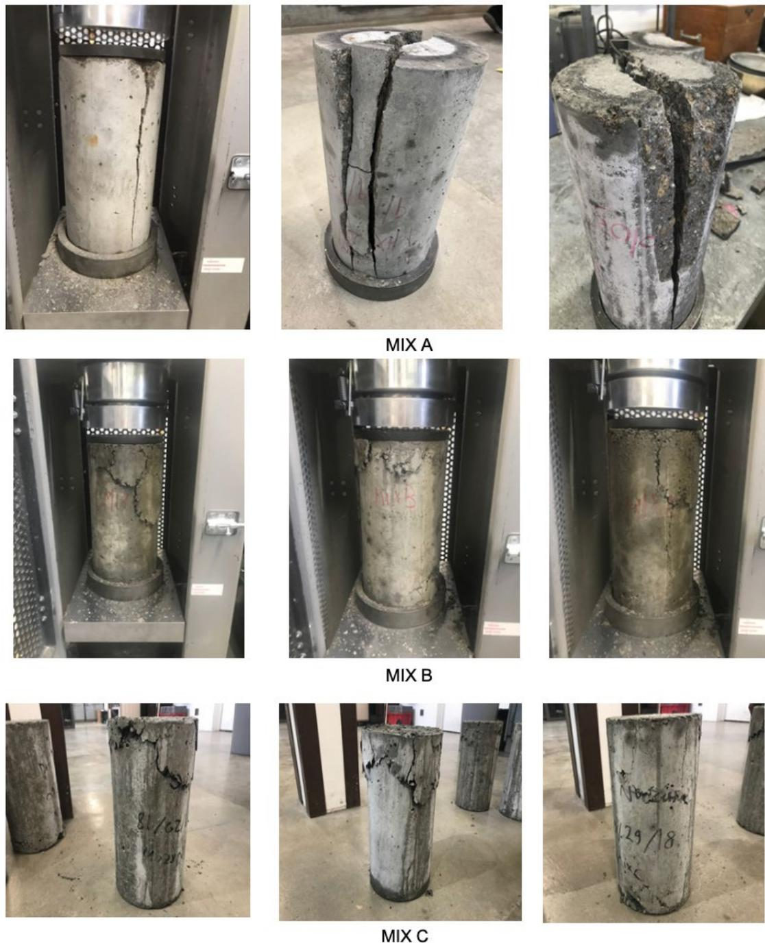
**Figure 12. Fracture Pattern in Cylindrical Specimens – Compression Test**
