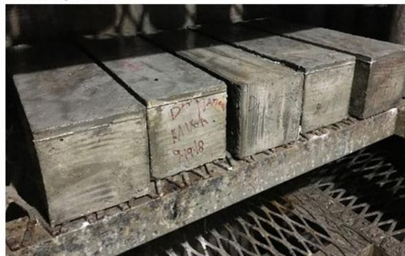
Beam specimens in the curing room
