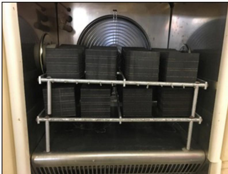
**Figure 3. FRBs Spaced Apart in Air Oven for Curing**
