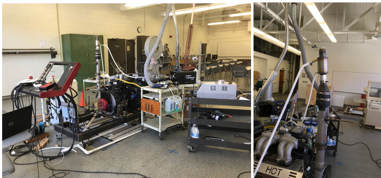
Figure 1. The Compressed Natural Gas (CNG) Engine with Humid Air System
