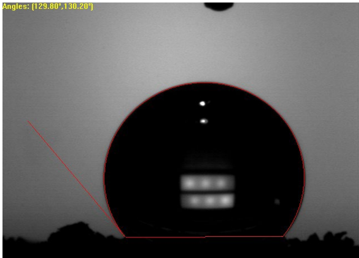
Figure 7. Contact Angle Measurement of Sample MD400
