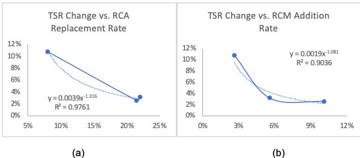
Figure 30. Relationship between TSR Change and RCA Replacement Rate or RCM Addition Rate
