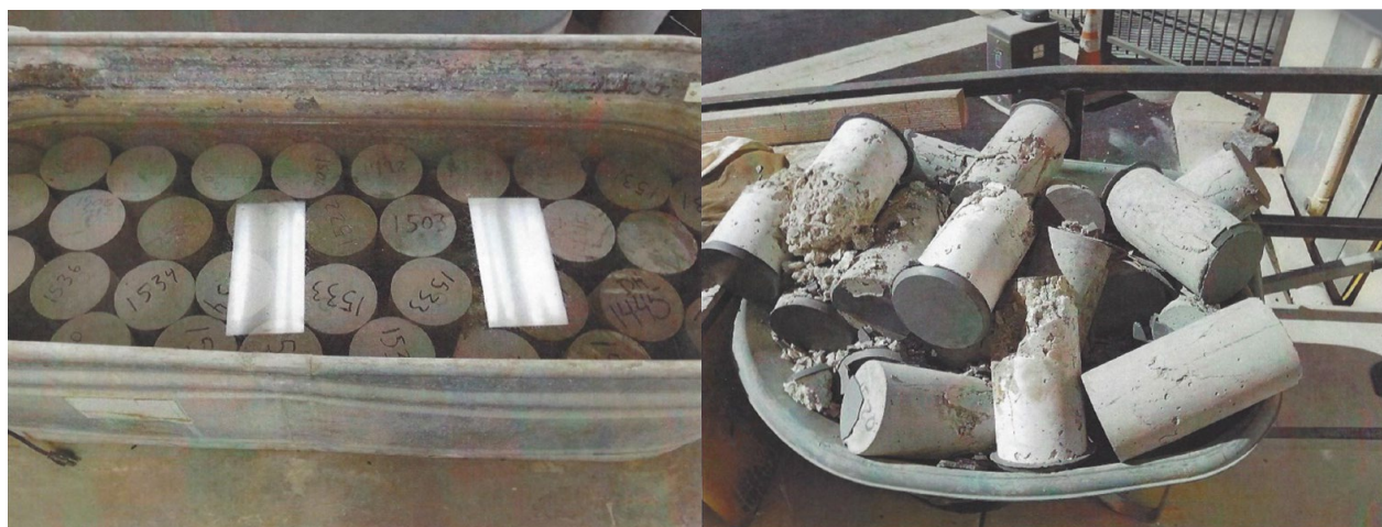
Figure 3. Concrete Cylinder for a Recent Bridge Pour Project
