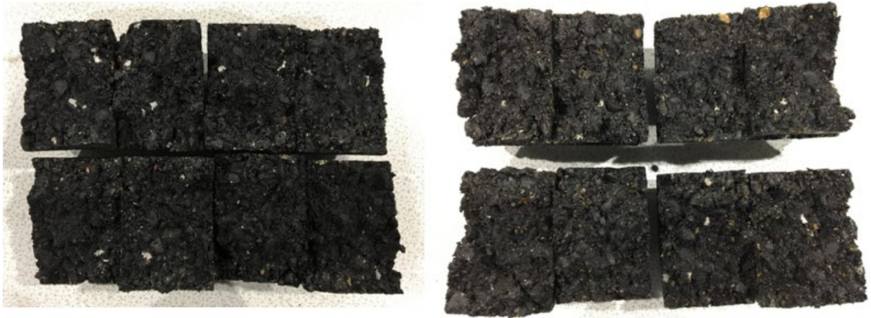
Figure Appendix C-2: AASHTO 283 Test Photos of RCA 9.5–12.5mm Mix. Left (Dry), Right (Wet)
