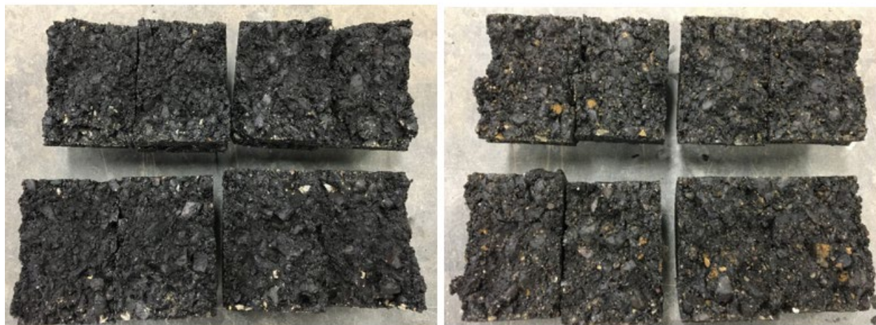
Figure Appendix C-1: AASHTO 283 Test Photos of Control HMA Mix (100% virgin aggregate). Left (Dry), Right (Wet)
