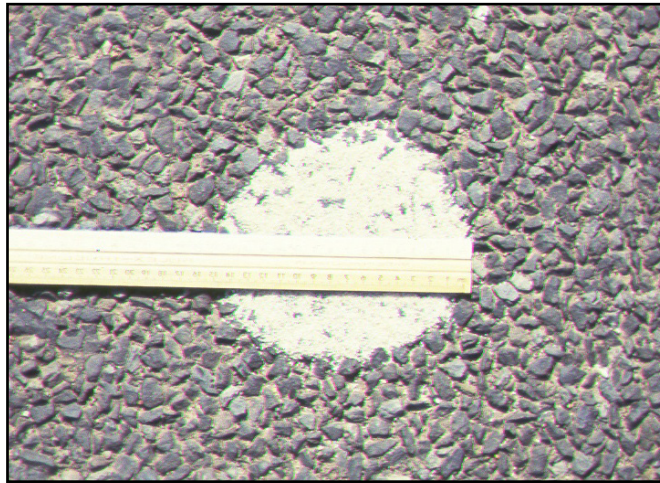
b) Sand Patch Test
