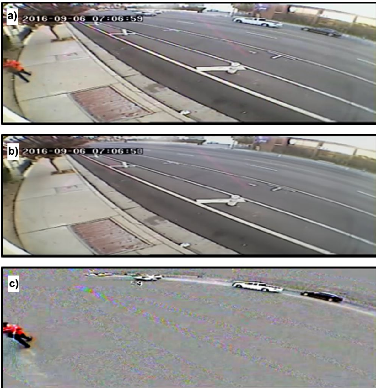
Figure 3. Background Subtraction: (a) Original Video Frame; (b) Estimated Background; and (c) Moving Objects After Background Subtraction
