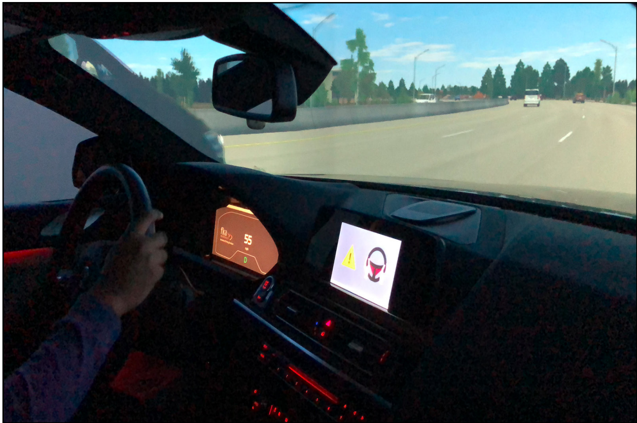
Figure 4. Inside View of the Vehicle with Dashboard and Central Console, Shown at the Time of Warning Display
