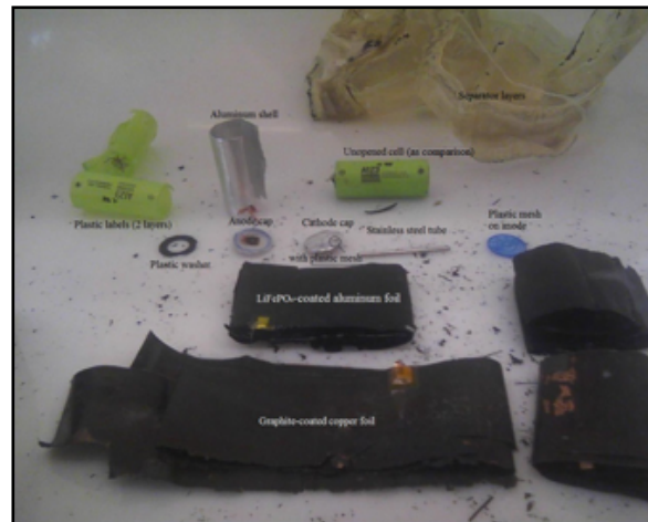
Layout of a Disassembled LiFePO 4 Cell with an Unopened Cell
