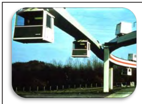
Figure 29. Cabintaxi Supported and Suspended Vehicles
