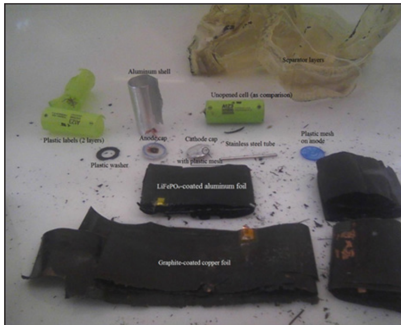
Layout of a Disassembled LiFePO 4 Cell with an Unopened Cell Source: Authors' photo, 2013.
