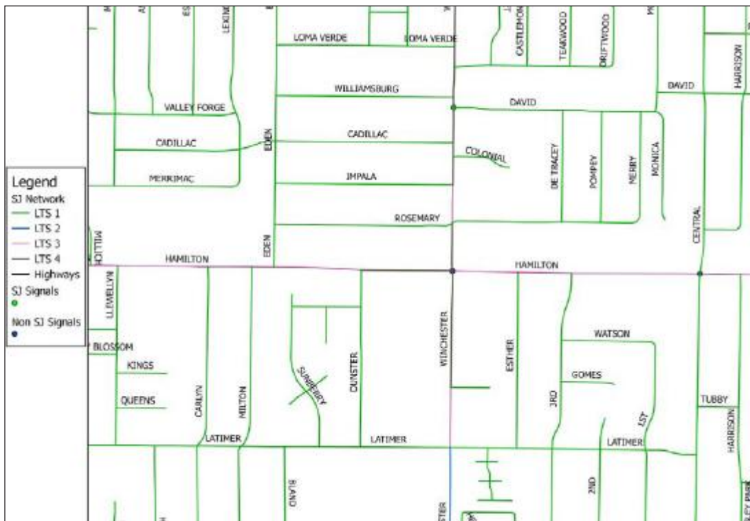
Figure 4. Stress Map Without Intersection Effect, Implying Low-Stress Routes Across Winchester Blvd. Using Rosemary Lane or Latimer St.
