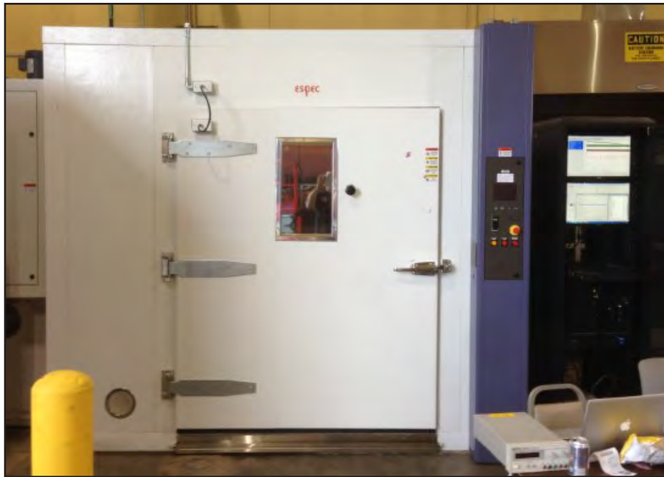
Figure 2. Temperature-Controlled Test Chamber
