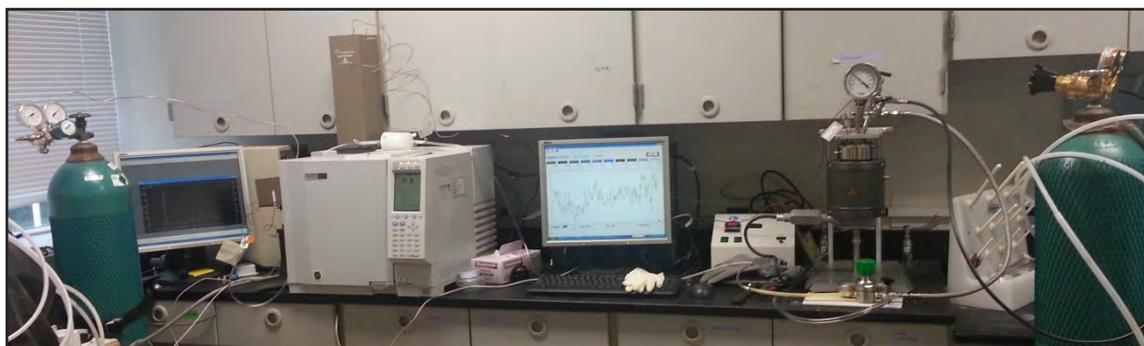
**Figure 7. GC Connected to the Reactor for Analyzing Emission Compositions**
